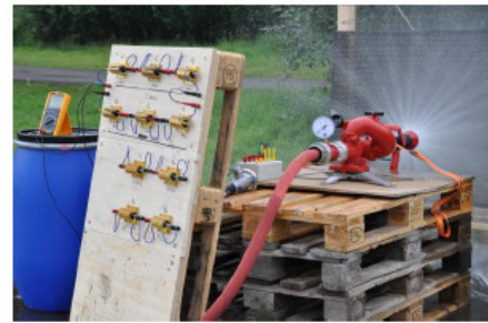
Figure 3: Testing conductivity of spray water jet at 1000V, TÜV Rheinland 2011
